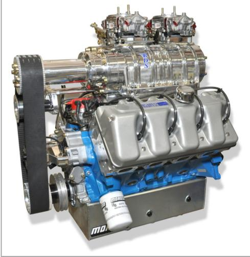
Seven months ago Jon Kaase introduced his new Boss Nine engine to much acclaim. Constructed with either a cast iron or cast aluminum block it was developed using five intake manifolds. These suit 4150- 4500- and Tunnel Ram-style carburetors, Keith Wilson's EFI conversion, and Hilborn's stack injection. But today's news is of their blower version.
