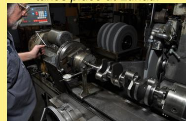
here Robert keeps a steady hand on the controls as he checks for run-out before grinding commences.
