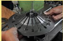
It was then Ram Clutches received a call for assistance. Two days later they had created a high-performance dual-disc assembly complete with lightweight flywheel, and all was well again. To ensure their high-performance clutches release fully before the fingers travel over-center, Ram employs a high-cone diaphragm. Ram also produces a high-performance single-plate replacement for Ford's latest 5.0 GT flyers.
