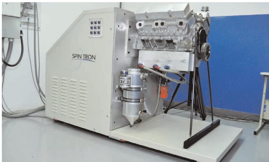
The Spintron uses a substitute crankshaft that powers the internal engine components as fast or as long as desired. It measures and records valve movement via laser tracking. Previously, it was assumed that valve timing was controlled by the shape of the camshaft lobe, but at higher engine speeds the Spintron quickly contradicted this theory as it had the ability to calculate the deflection of a pushrod and measure the loss of contact between the camshaft and the valve train.
