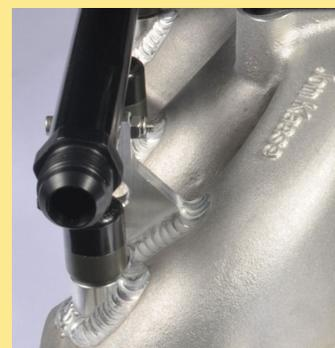
Two of the chief difficulties in converting to fuel injection are the installation (and the exact placement) of injector bosses and the installation of the fuel rail stanchions. Today's news reveals Wilson Manifolds' convenient new service to help engine builders and racers—a rapid turnaround service that accomplishes this and more.
