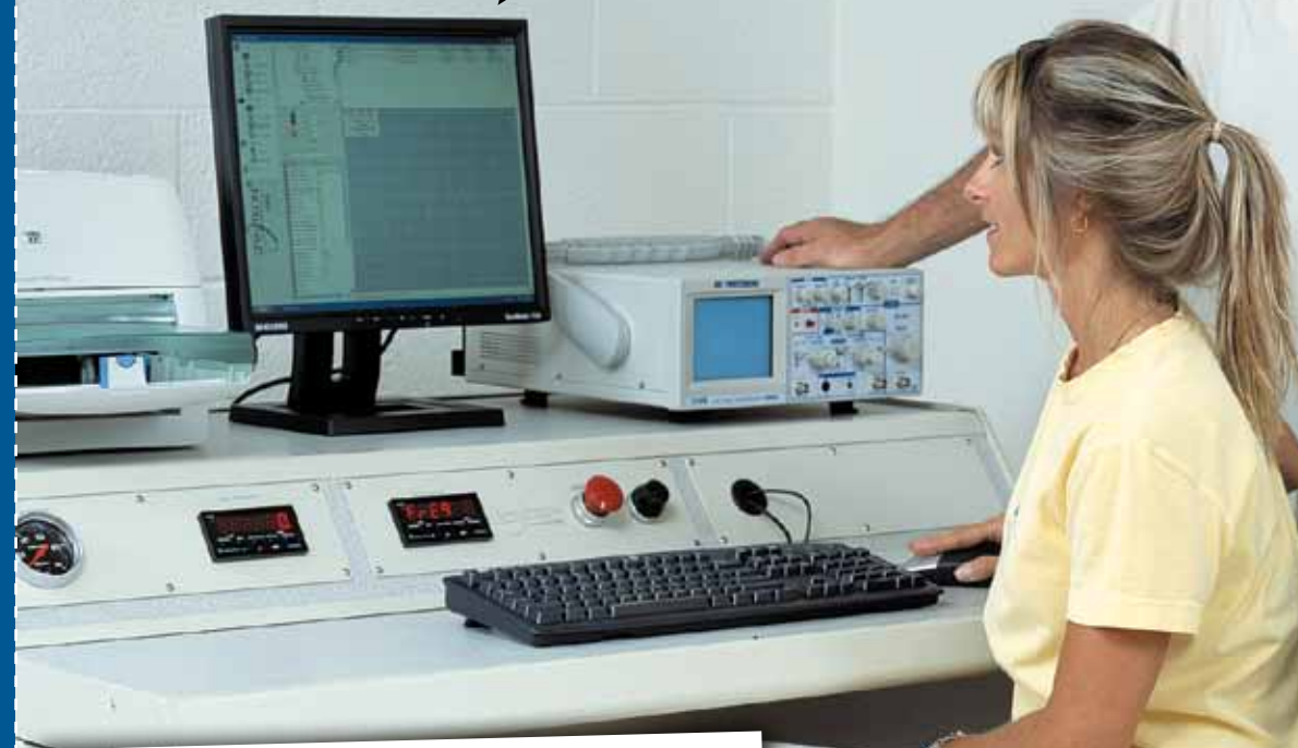
The apparatus on top of the SpinTron's console (under the gentleman's right hand) is an optional oscilloscope. Although the oscilloscope does not portray a baseline valve trace, it does verify the accuracy of the information transmitted to the computer via the LVTS.
