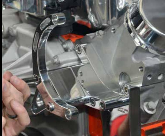
■ **CNC-machined brackets make the case for the well-designed kit. You don't want to have to ruin the finish and risk weakening your parts by grinding and tweaking to make them fit.**
