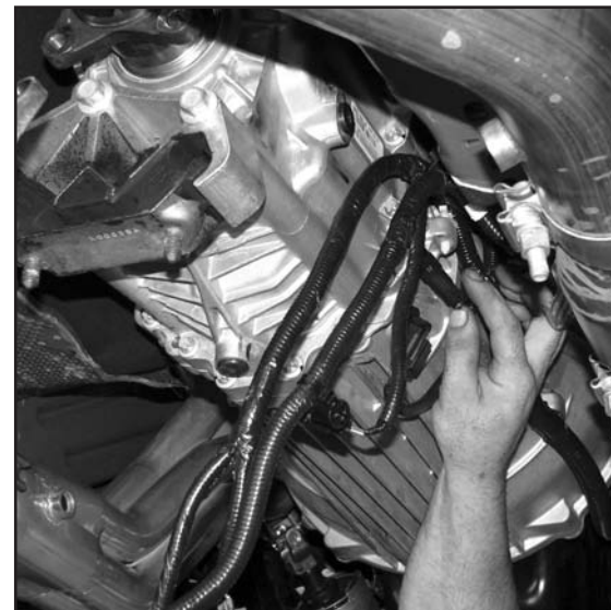
>> With the big job completed, attention turned to hooking up the ancillaries such as these Medusa-like wire bundles and reattaching the clutch hydraulics. LaMotta followed this with the re-installation of the shift linkage, starter motor, the drive-shaft center support bearing, the featherweight aluminum cross-member, the front U-joint flange, the lower and upper chassis braces, and the rear U-joint flange.
