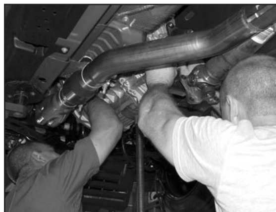
>> It took two big guys to wrestle the transmission back into place. The extension jack gave support while LaMotta tightened the bottom bellhousing bolts. Aftermarket exhaust headers on this car take up more room than the OE exhaust and made the job a little tougher.
