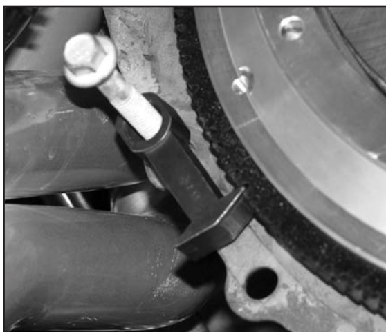
>> This simple but critical wedge bolts to the block and situates between the ring gear teeth of the flywheel preventing it from turning while bolts are being removed or tightened.
