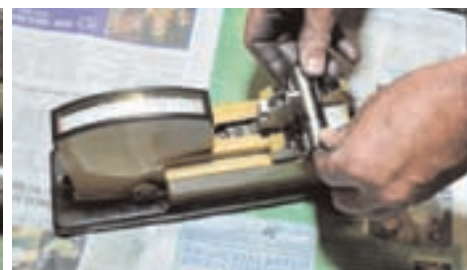
Piston pins are checked for straightness, and run-out is measured to 0.0001-inch. The run-out on the average pin is usually around this figure; if the indicator shows run-out of 0.0005-inch the pin will be renewed.
