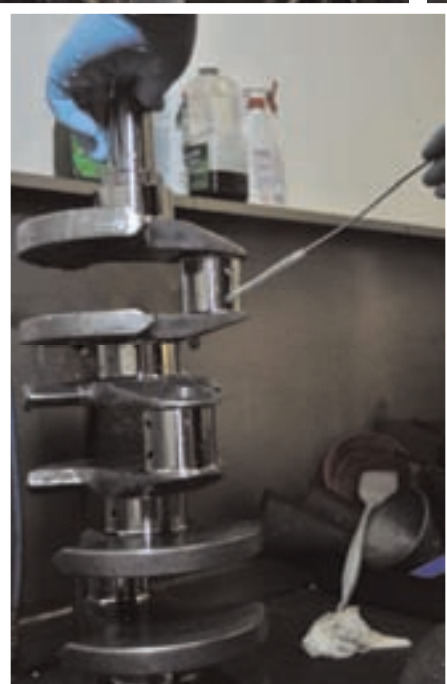
The engine is dismantled and the crankshaft is removed, cleaned and Magnaflux tested.
