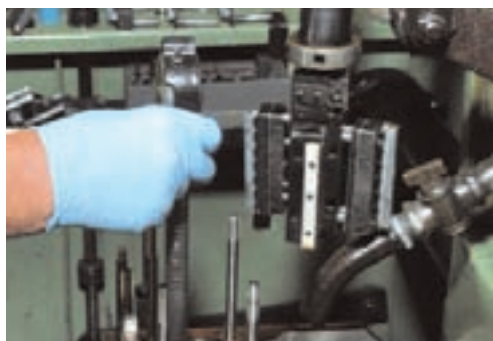
The art of cylinder honing is never taken more seriously than at Kaase's. It is the key to gaining a power output edge while maintaining a fine, consistent pattern of crosshatch scratches that lubricates the rings.
