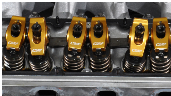
The P38 operates with slightly altered intake valve pockets on the piston crowns, narrow stud-style rockers, appropriate guide plates, and different valve covers.
